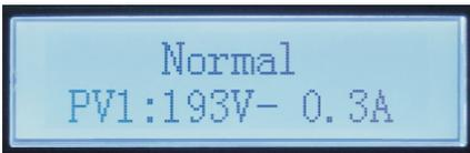
2.Inverter working status, PV generated power
